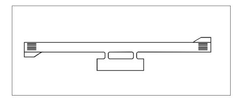
Figure 3-1. Typical turn pad layout
