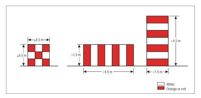
Figure 6-1. Basic marking patterns
