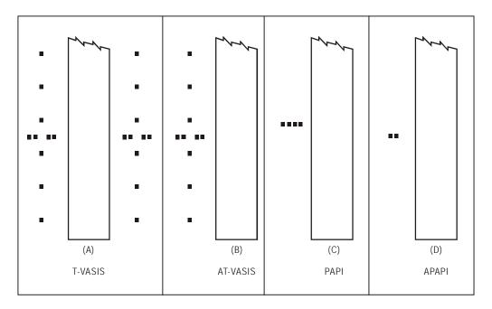
Figure 5-16. Visual approach slope indicator systems
