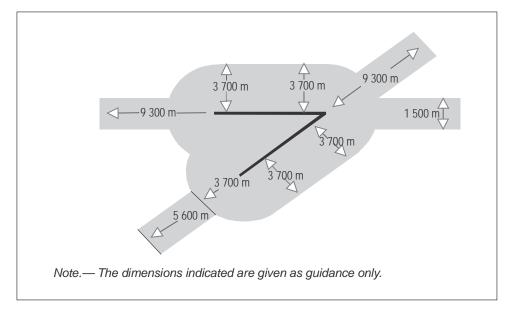
Figure 5-12. Multiple runway laser-beam free flight zone
