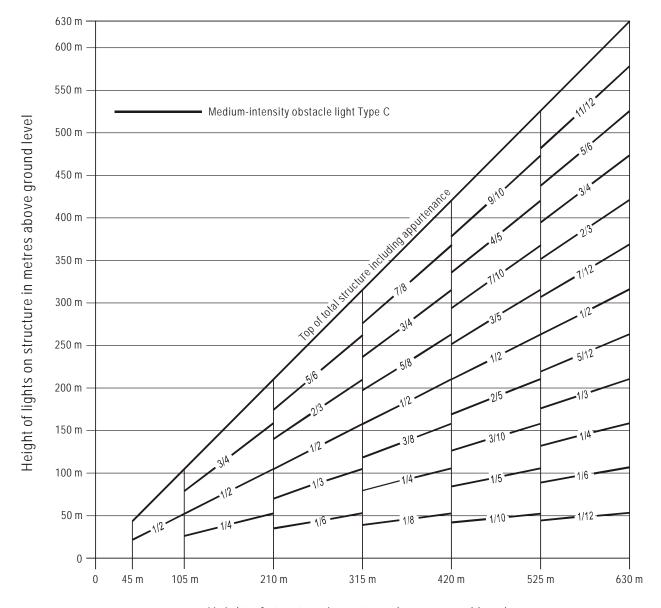
Height of structure in metres above ground level
