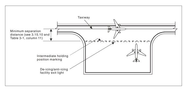
Figure 5-28. Typical remote de-icing/anti-icing facility
