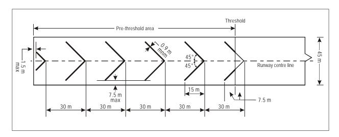
Figure 7-2. Pre-threshold marking
