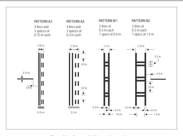
Figure 5-8. Runway-holding position markings
