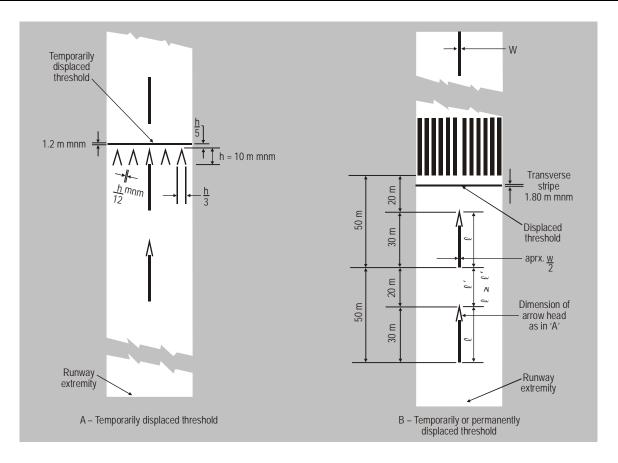
Figure 5-4. Displaced threshold markings
