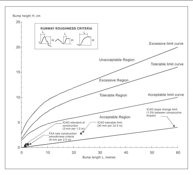
Figure A-3. Comparison of roughness criteria
