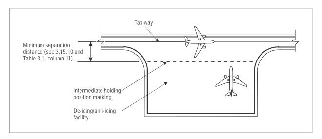
Figure 3-4. Minimum separation distance on a de-icing/anti-icing facility
