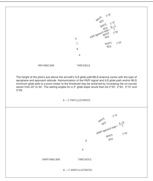
Figure 5-20. Light beams and angle of elevation setting of PAPI and APAPI
