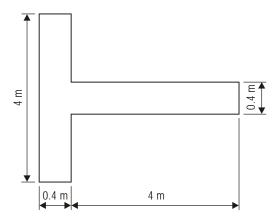
Figure 5-1. Landing direction indicator
